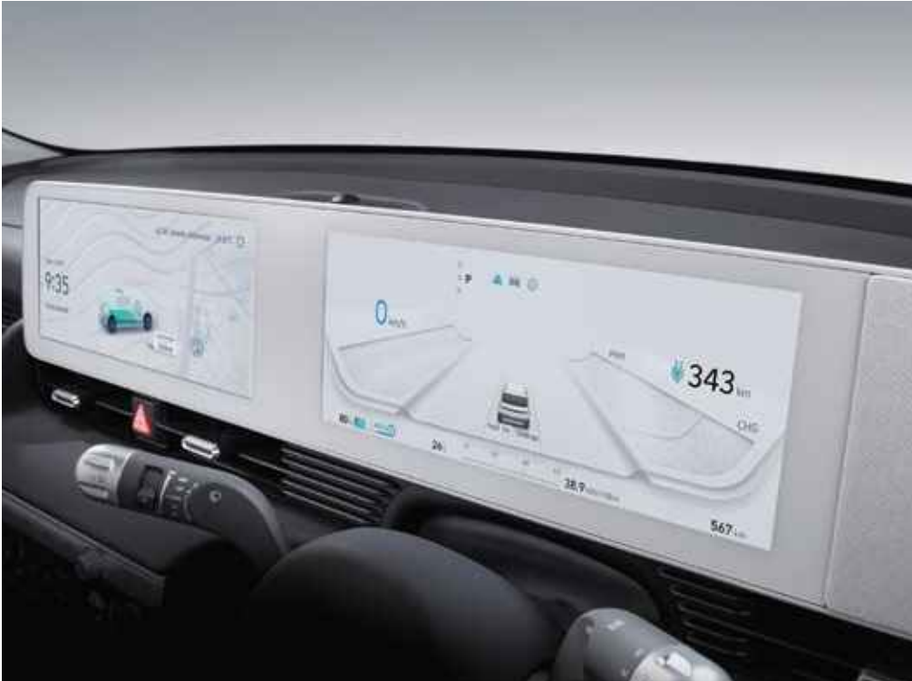
12.3" TFT LCD Cluster with integrated A/V System
