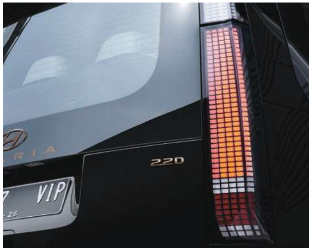
Parametric Pixel Light (LED Rear Combination Lamps)
