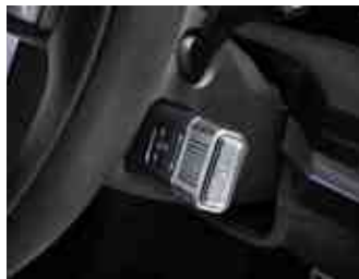
Column-type Shift by Wire (SBW)
