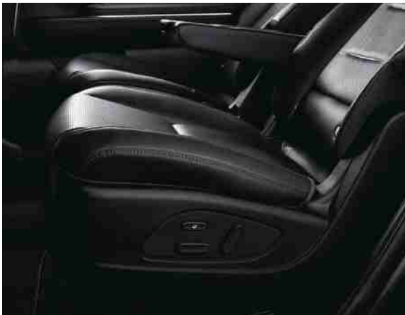
2nd and 3rd-row Remote Folding Switches 6-way Power 2nd-row Seats
