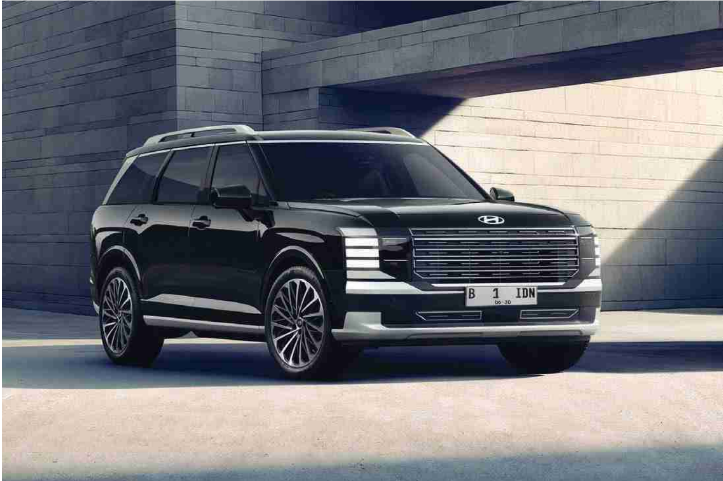
LED Projector Headlamps with hidden type LED Daytime Running Light (DRL) and Position Lamps
